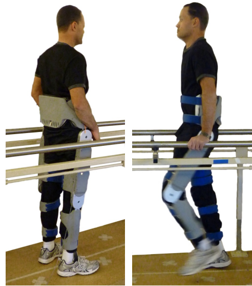
Fig. 7. Subject with T10 complete spinal cord injury walking wearing the powered orthosis.
